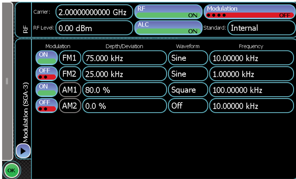
Typical multiple modulation set-up
